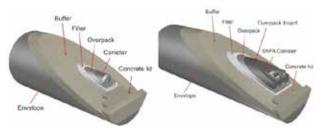
Figure 11 — Supercontainer for vitrifed high-level-waste (left) and UOX irradiated fuel (right)
