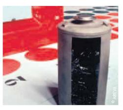
Figure 2 – Vitrified high-level metallic waste container
