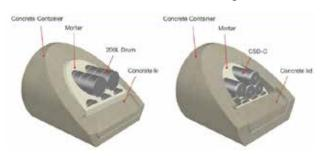
Figure 13 — Monolith B for category B waste (200 L drums) (left) and CSD-C (right)
