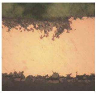
Light optical cross-section of a green area seen in the left flask above of the initially 100 $\mu$ m metallic copper foil after 15 years exposure in distilled water. Localised corrosion attack is clearly visible.
