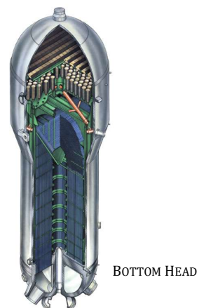
FIGURE 5A TYPICAL STEAM GENERATOR
